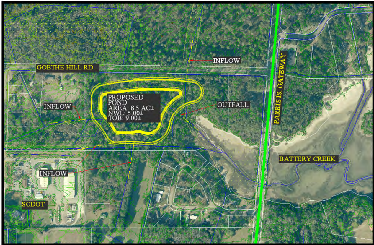
Figure 5-6 - Grober Hill M2 Proposed Regional Pond Layout
