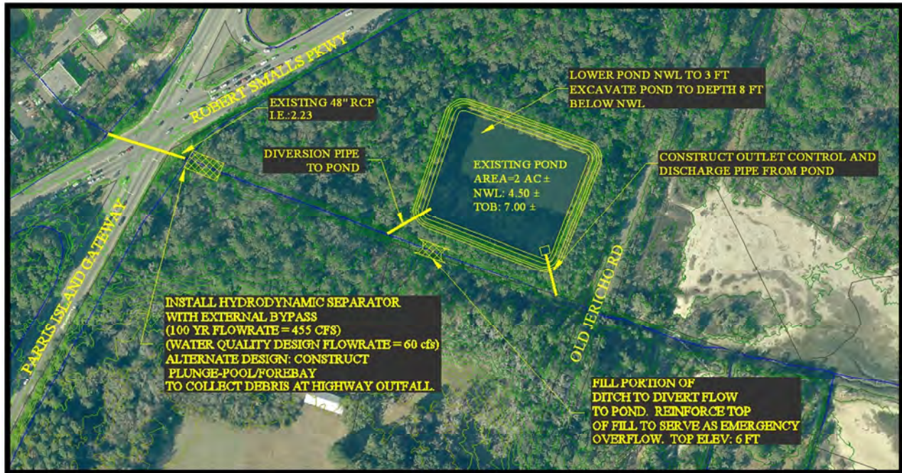
Figure 5-9 - Burton Hill M2 Proposed Regional Retrofit Layout
